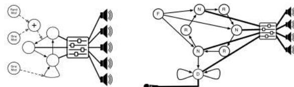
Figure 3. Network topologies for the pieces *Roj* (left) and *Errant it is* (right). The labels stand for: F = Fourses unit, N = Izhikevich neuron, R = Karplus-Strong resonator, D = feedback and delay unit.
