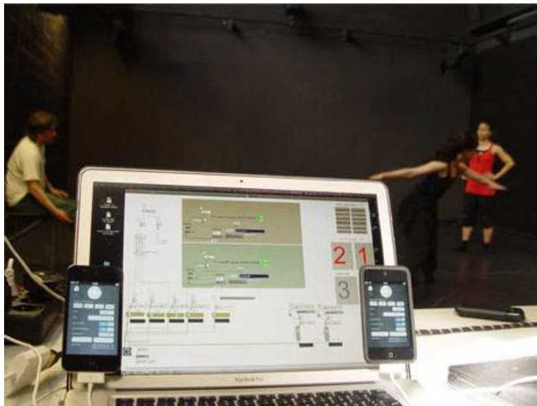
Figure A4. The software Choreophony . The photograph (copyright by Chris Ziegler) shows the software Choreophony running on a laptop together with two iPods which are being used as acceleration sensors for a dance rehearsal.
